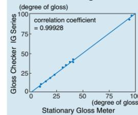
The above graph shows the results of measuring ceramic tiles, widely used as the standard surface for the medium-gloss range (secondary standard surface) because of the stability of surface conditions. The IG Series produces extremely precise values.
